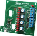
The KBMG Multi-Speed Board provides 4-user selectable preset speeds to control a motor connected to the KBMG Series Regenerative Drive. A preset (PS 1, PS 2, PS 3, PS 4) is selected with a contact closure or open collector. Motor direction is set by the position of Jumper R/F (reverse/forward) which is provided for each preset. Connections to the Multi-Speed Board are made with a barrier terminal block. A connector is available for a tach-generator, if required.
